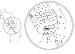
Connect the charger to a power source and the micro USB connector to the port at the base of the phone, under the USB/audio protective cover.
